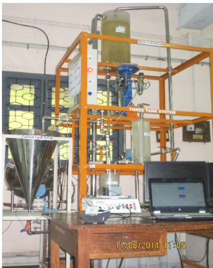
Fig. 2. Experimental setup of a conical tank process.
