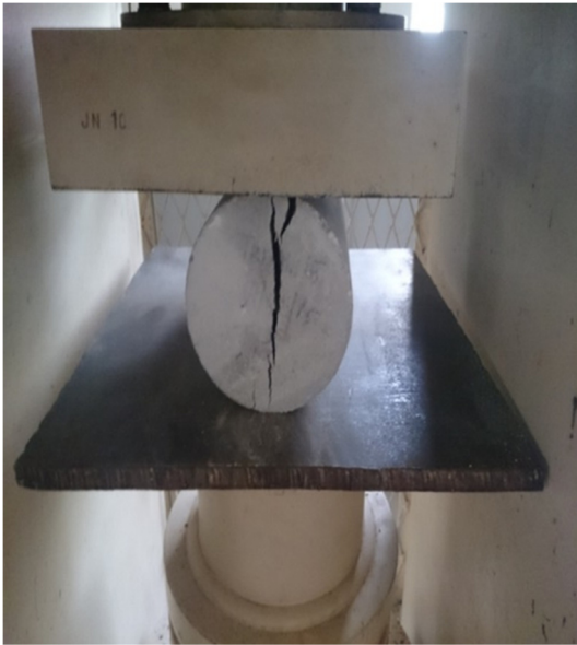
Fig. 9. Split tensile strength testing.
