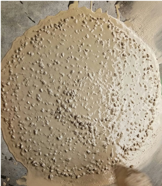
Fig. 5. Flow of SCC control mix.
