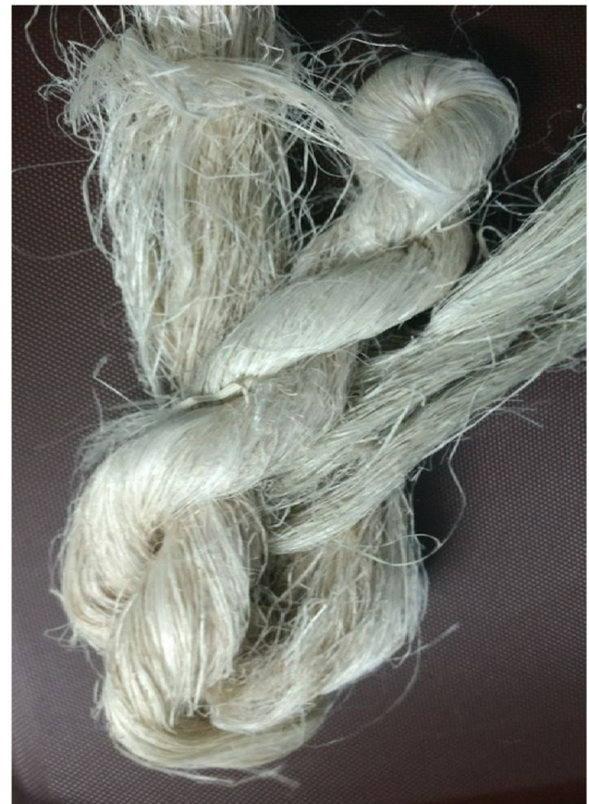
Fig. 3. Long Sisal Fibres procured for experiment.
