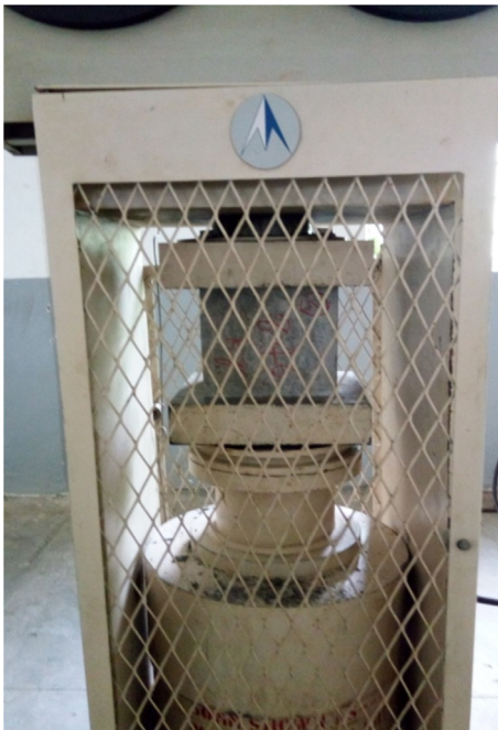
Fig. 6. Cube testing by compression testing machine.
