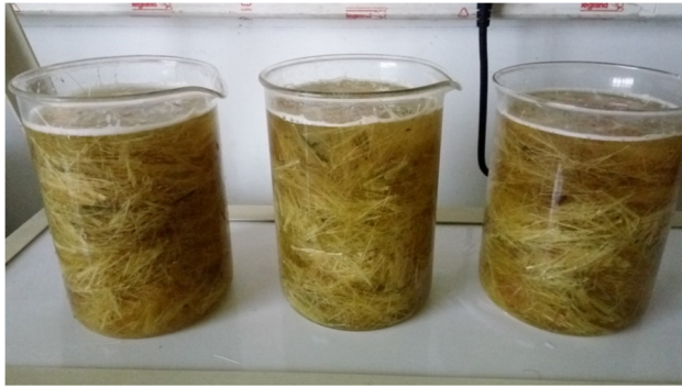
Fig. 4. Fibres cut into 25 mm length kept for alkali treatment with 4% NaOH.
