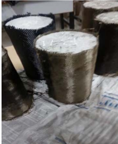
Figure 1. Concrete test cylinders wrapped with Basalt Fibre
