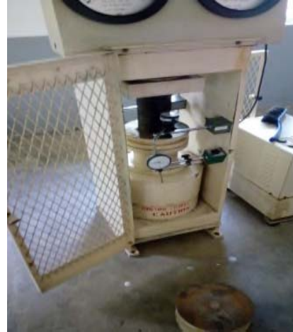
Figure 2. Testing of Basalt specimen in Compression Testing machine
