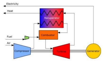
Microturbines are small and simple-cycle gas turbines.
